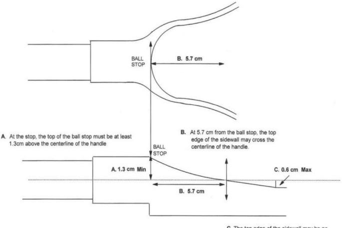
C. The top edge of the sidewall may be no more than .6 cm below the centerline of the handle
