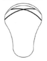
Two separate throw strings; One horizontal across upper third of the head; one inverted "U" in upper one-half of head.
