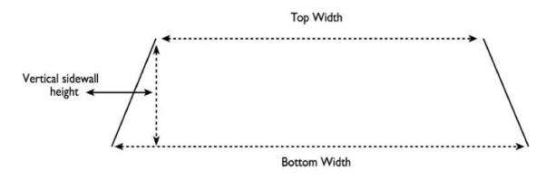
Bottom Width — Top Width = < 0.65cm Vertical Sidewall Height
