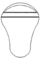
Two separate horizontal throw strings; both attached in upper third of the head
