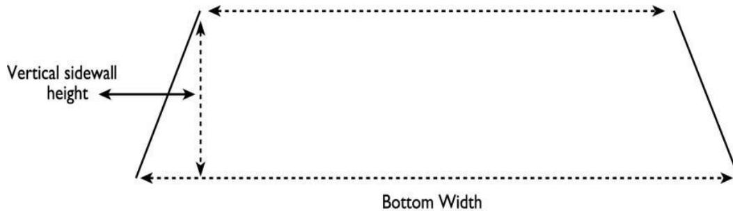
$$\frac{\text{Bottom Width} - \text{Top Width}}{\text{Vertical Sidewall Height}} < 0.50$$
